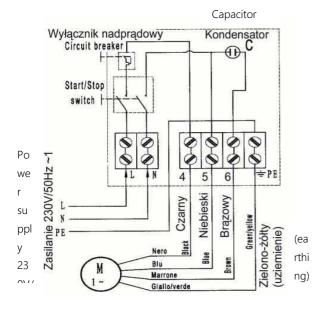
The cable box is separately delivered to some types of pumps. There is a starting capacitor built in the cable box as well as an overcurrent protection, switch. The picture presents the diagram of cable core connection of the power supply cable to the connecting strip in the box. Cable cores of the power supply cable are marked with small tags with core no. When identifying cores with tags or colour, connect them according to the diagram.
