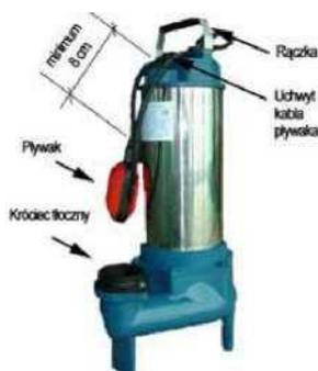
Min. dimensions of the drained tank should allow the float to freely move around in the pumped liquid, concurrently, not touching the tank walls. If there is a hazard that the float can get attached to the tank wall, the pump operation should be subject to direct supervision of the user so that there is no failure connected with potential “dry” operation.
